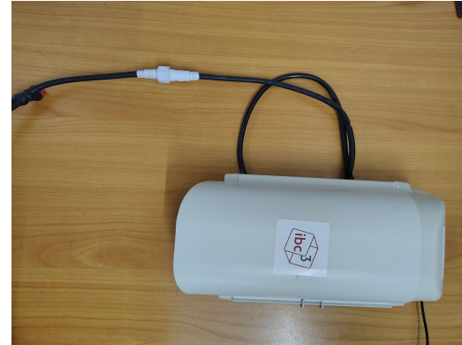
Step 2 : Connection of the adapter from the battery after 10 seconds
